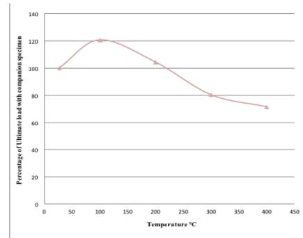
Fig. 8 Variation of ultimate load in percentage with companion specimen with Temperatures from 27 to 400°C for RCC Columns with 1.0 % steel fibers
