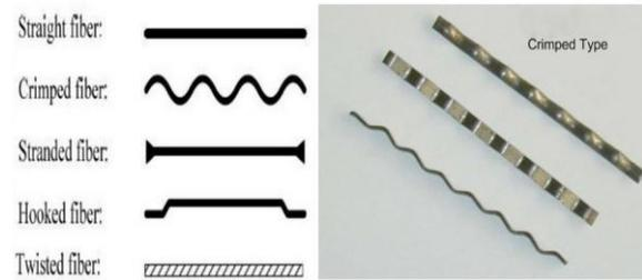
Fig.1 Types of steel fibers
