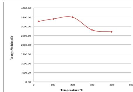
Fig. 11 Variation of Young's Modulus with Temperatures for RCC Columns with 1 percent steel fibers
