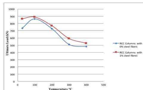
Fig. 9 Variation of Ultimate loads of RC Columns with Temperatures from 27 to 400°C without steel fibers and with 1% steel fibers
