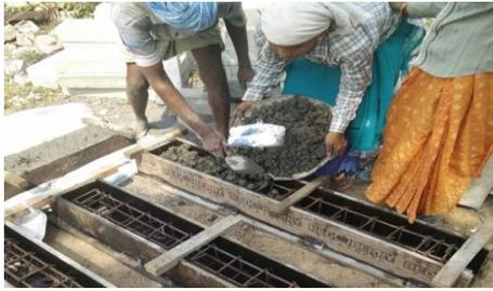
Fig. 2 Reinforcement cage placed in moulds
