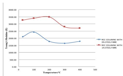
Fig.12 Variation of Young's Modulus with temperatures for RCC Columns without and with steel fibers
