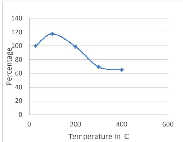
Fig.7 Variation of ultimate load in percentage with companion specimen load with Temperatures from 27°C to 400°C for RCC Columns without steel fibers
