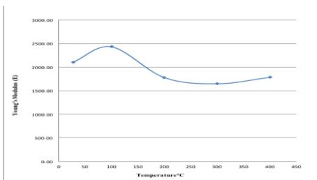
Fig.10 Variation of Young's Modulus with Temperatures from 27 to 400°C of RCC Columns without steel fibers
