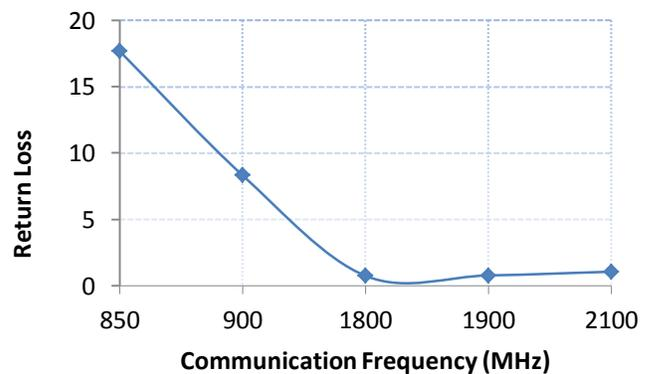
Figure 5.2 Variation in Return Loss with varying frequencies
