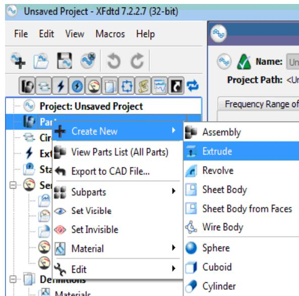
Figure 4.2: Selecting the geometry tool to perform an extrusion
