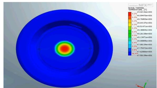
Fig.7. Heat Flow Simulation of New Al (Inside Module)
