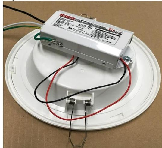
Fig.1. LED Module Case with No Heatsink
