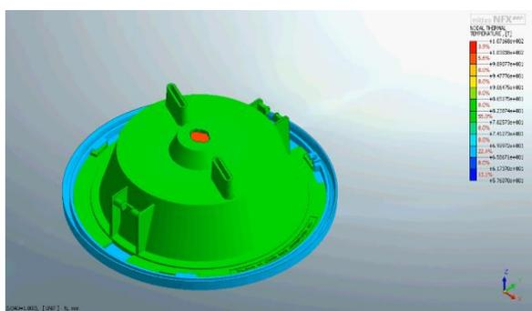
Fig.10. Heat Flow Simulation of Cu (Outside Module)
