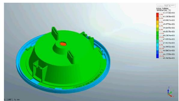
Fig.6. Heat Flow Simulation of Al (Outside Module)
