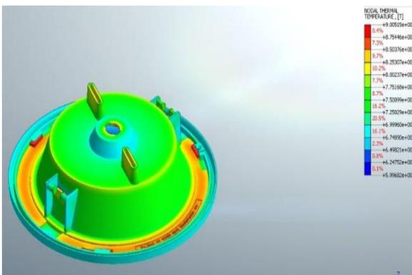
Fig.4. Heat Flow Simulation of PC (Outside Module)
