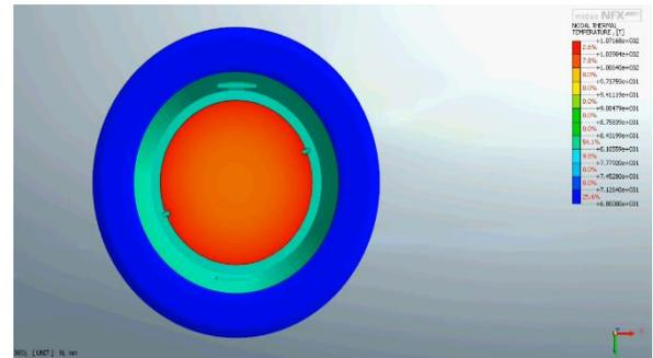
Fig.5. Heat Flow Simulation of Al (Inside Module)
