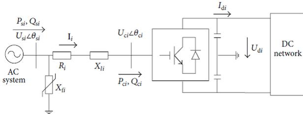
Fig. 1 Simplified circuit diagram of single-phase VSC-HVDC.
