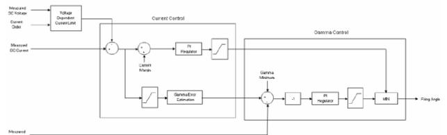
Fig. 2 Block Diagram of Converter Controller
