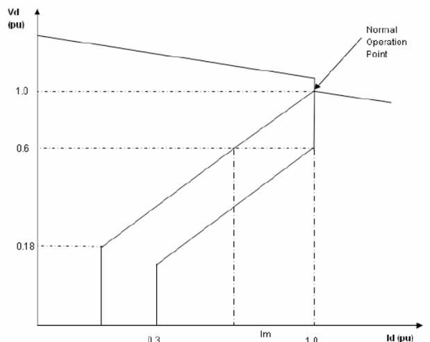
Fig. 3 Voltage Dependent Current Order Limits Used in the Converter Control Scheme
