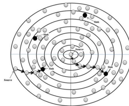
Fig13: Illustration of data packets development towards the random sink placement.
