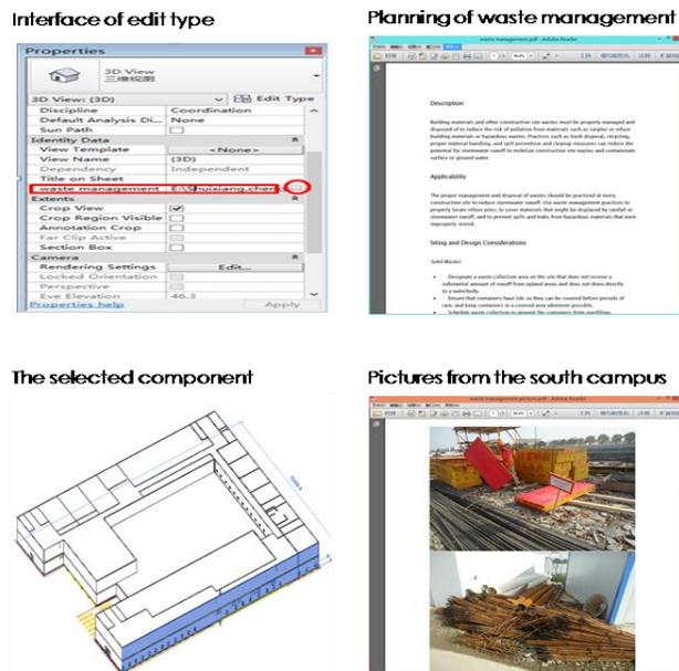
Fig. 10 Waste Management integrated in the BIM model
