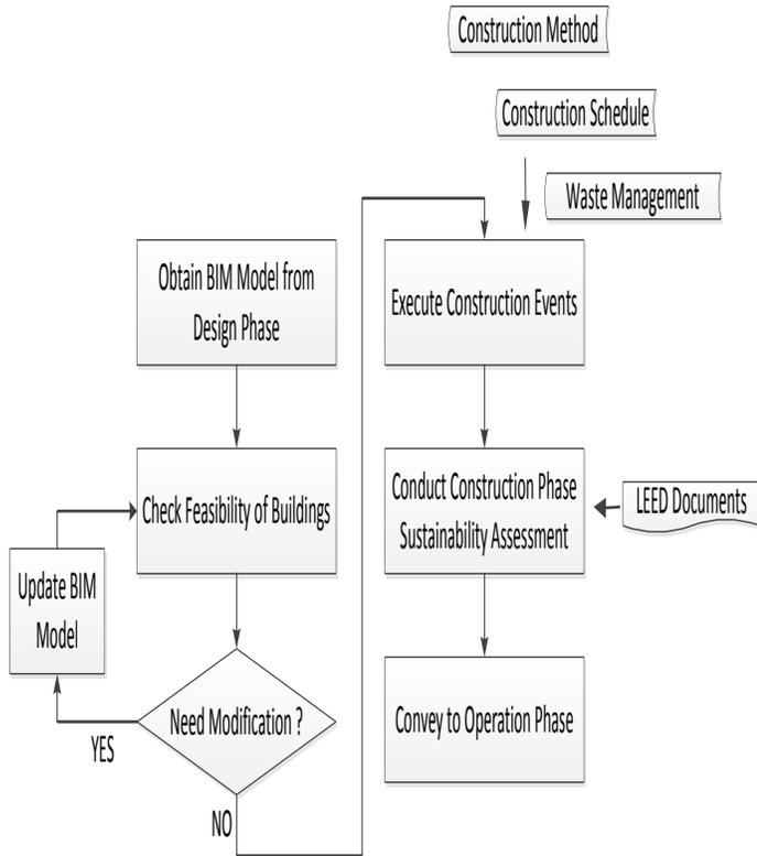
Fig. 1 Framework of sustainability assessment during construction stage
