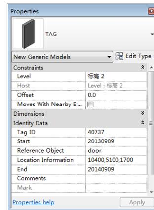
Fig. 4 RFID Data Representation in Properties
