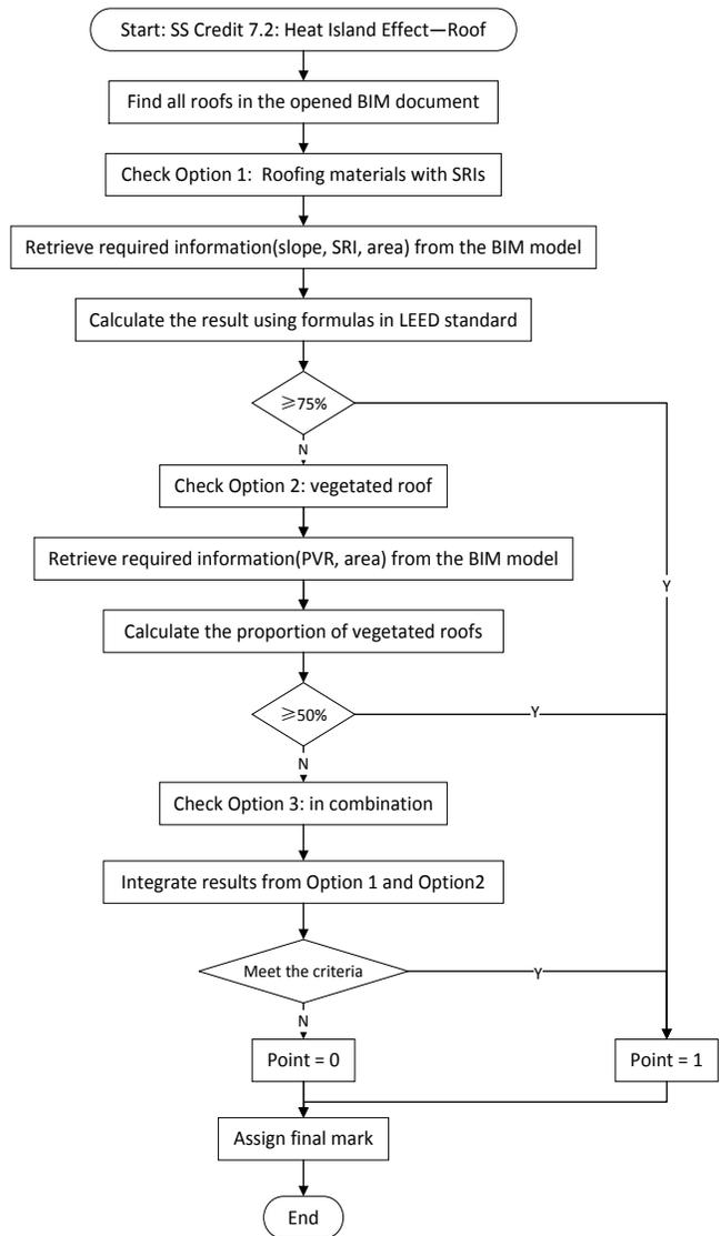
Fig. 2 Example of a rule-based assessment
