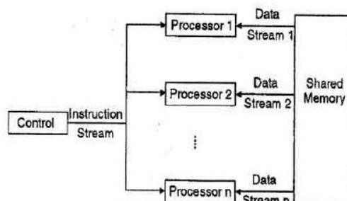
MIMD is the most powerful computer system MIMD computers are consisting of 'n' processing units and each with its own stream of instruction. MIMD covers the range of multiprocessor systems. The block diagram of MIMD computer is shown.
