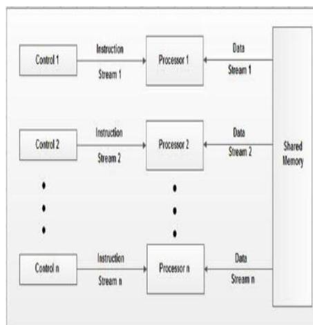
A parallel computer is a set of processors that are able to work to solve a computational problem.
